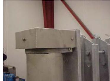
1. Remove both hats with a 10 mm open-ended spanner.
