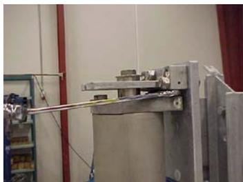
4. Adjust the screws to the required height which is obtained when the fronts of the forks are 12 mm above the front beam of the freezer. Take care that the lifting beam is still parallel to the rear side of the forks. Use a 24 mm open-ended spanner.
