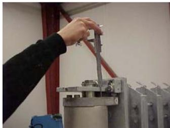
2. Measure distance between supporting plate and hanging plate both at front and rear.
