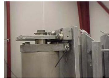
3. Release the locking screws with a 3mm hex key.
